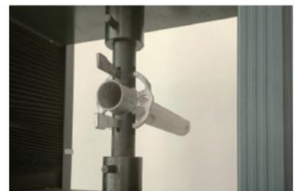
Tensile Strength Test Maximum tensile strength Rosettes can withstand during the stretching process
